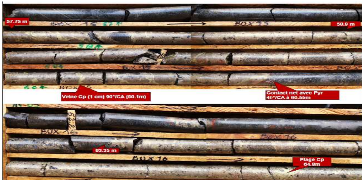
Figure 4: Hole SM44-428267 intersected 54 m of mineralized pyroxenite, grading 0.96% nickel, 0.76% copper and 0.74 gpt palladium, including a combined 8.0 m of massive sulphide grading 4.08% nickel, 2.43% copper & 2.92 gpt palladium at the Samapleu Main deposit.
