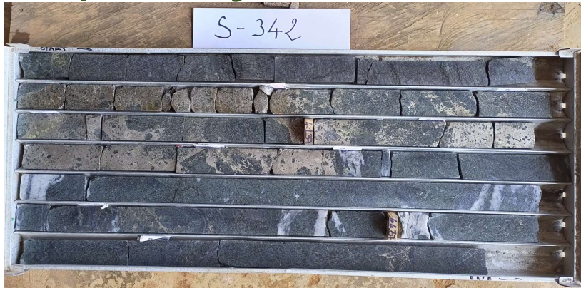
Hole S-342 returning a 38 m thick mineralised magmatic pyroxenite with a 4.35 m of massive sulphide grading 1.58% Ni and 0.65% Cu.
