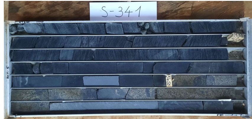
Hole S-341 showing massive sulphide lenses within a 21 m thick magmatic pyroxenite including 2.75 m of massive sulphide at 1.02% Ni and 0.56% Cu.
