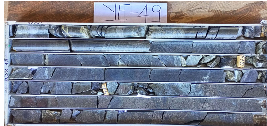
Hole Y-49 returning 14 m of mineralized gabbroic intrusive with 10.95 m at 0.58% Ni and 0.80% Cu including 5.55 m grading 0.95% Ni and 1.37% Cu is confirming the presence of a second mineralised zone. Individual values reach up to 3.41% Cu (103.20 m) and 1.53% Ni (99.50 m).
