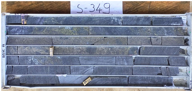
Hole S-349 intersecting a 53 m of combined mineralisation layers grading 0.29% Ni including 2.60 m at 1.31% Ni and 0.95% Cu. The photo is showing a 1.65 m semi-massive to massive mineralisation grading 1.63% Ni and 0.63% Cu from 73.20 m to 74.85 m vertically from surface.
