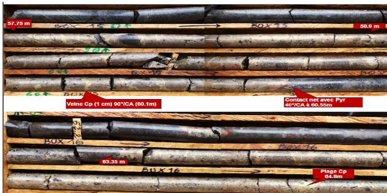
Figure 4: Hole SM44-428267 intersected 54 m of mineralized pyroxenite, grading 0.96% Ni, 0.76% Cu and 0.74 gpt palladium, including a combined 8.0 m of massive sulphide grading 4.08% Ni, 2.43% Cu & 2.92 gpt palladium at the Samapleu Main deposit.
